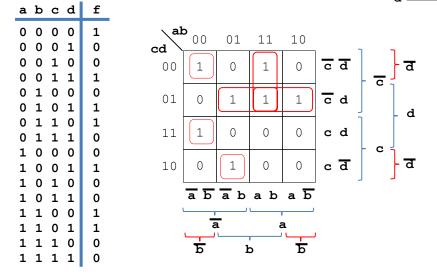
$f = \bar{a}\bar{b}\bar{c}\bar{d} + \bar{a}\bar{b}cd + \bar{a}bc\bar{d} + ab\bar{c} + a\bar{c}d + b\bar{c}d = \bar{a}\bar{b}(\overline{c\oplus d}) + \bar{a}bc\bar{d} + ab\bar{c} + \bar{c}d(a+b)$
