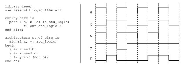
b) The following is the timing diagram of a logic circuit with 3 inputs. Sketch the logic circuit that generates this waveform. Then, complete the VHDL code. (10 pts)
